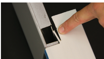
TAB BENT SUCCESSFULLY
